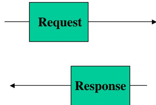
**Bus occupied until “Response” is returned. Bus can not be released until the request and response phase completed.**
