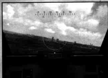
Missile seeker tracking a target with a radar lock, but outside of launch parameters.
