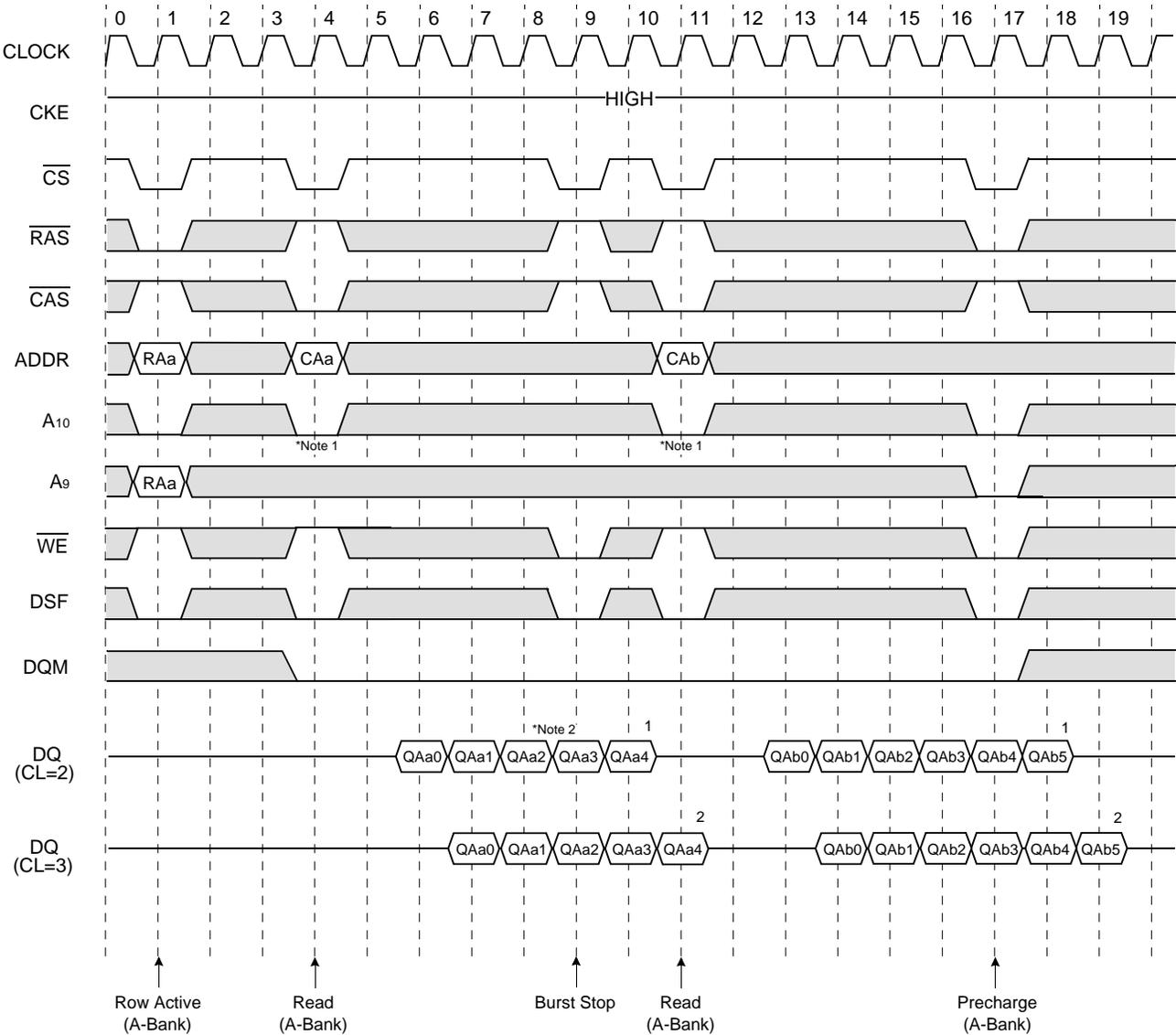
**\*Note :** 1. At full page mode, burst is wrap-around at the end of burst. So auto precharge is impossible.
