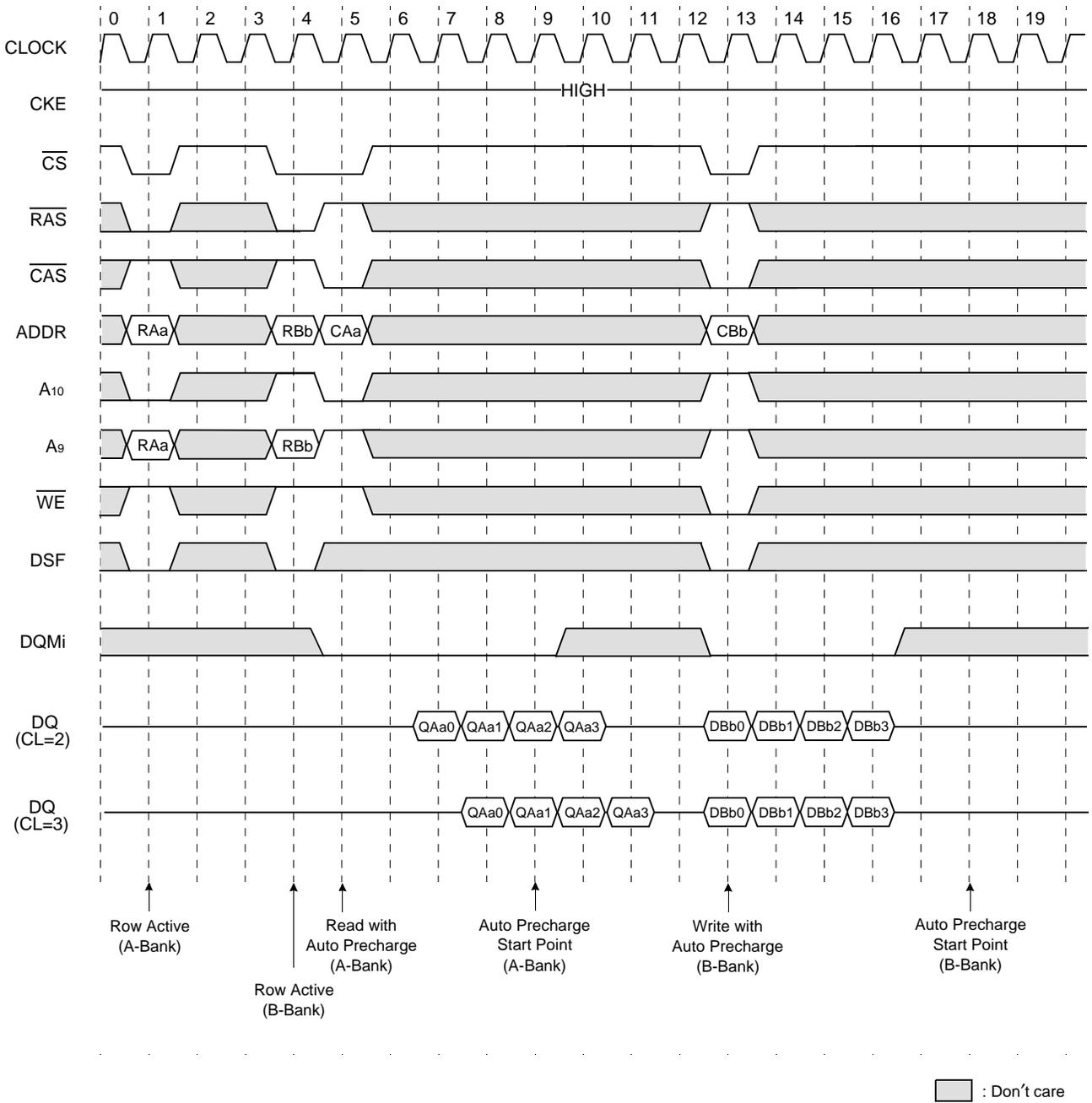
\*Note : 1. t<sub>RC</sub>D should be controlled to meet minimum t<sub>RA</sub>S before internal precharge start.
