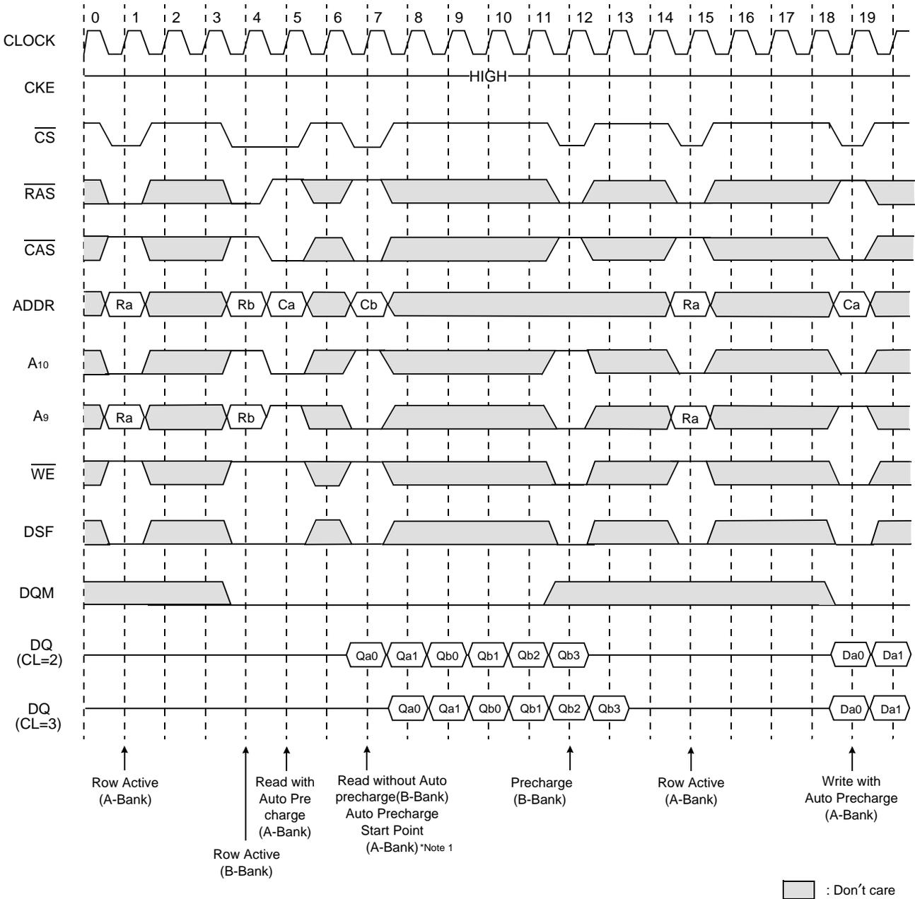
**\*Note:** 1. When Read(Write) command with auto precharge is issued at A-Bank after A and B Bank activation.
