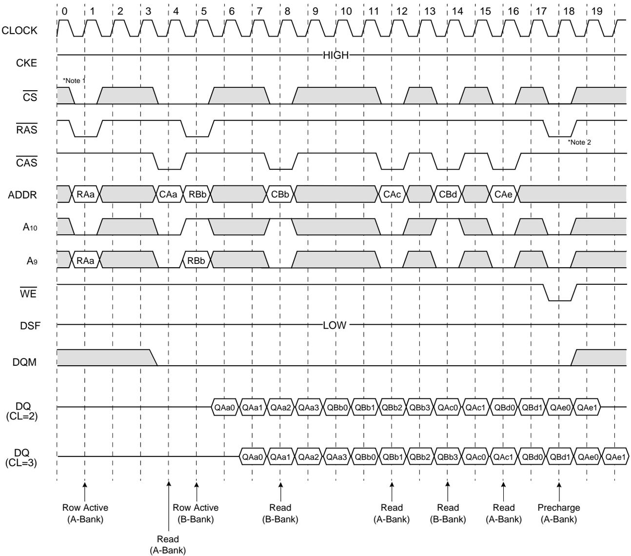
\*Note : 1.  $\overline{CS}$  can be don't care when  $\overline{RAS}$ ,  $\overline{CAS}$  and  $\overline{WE}$  are high at the clock high going edge.
