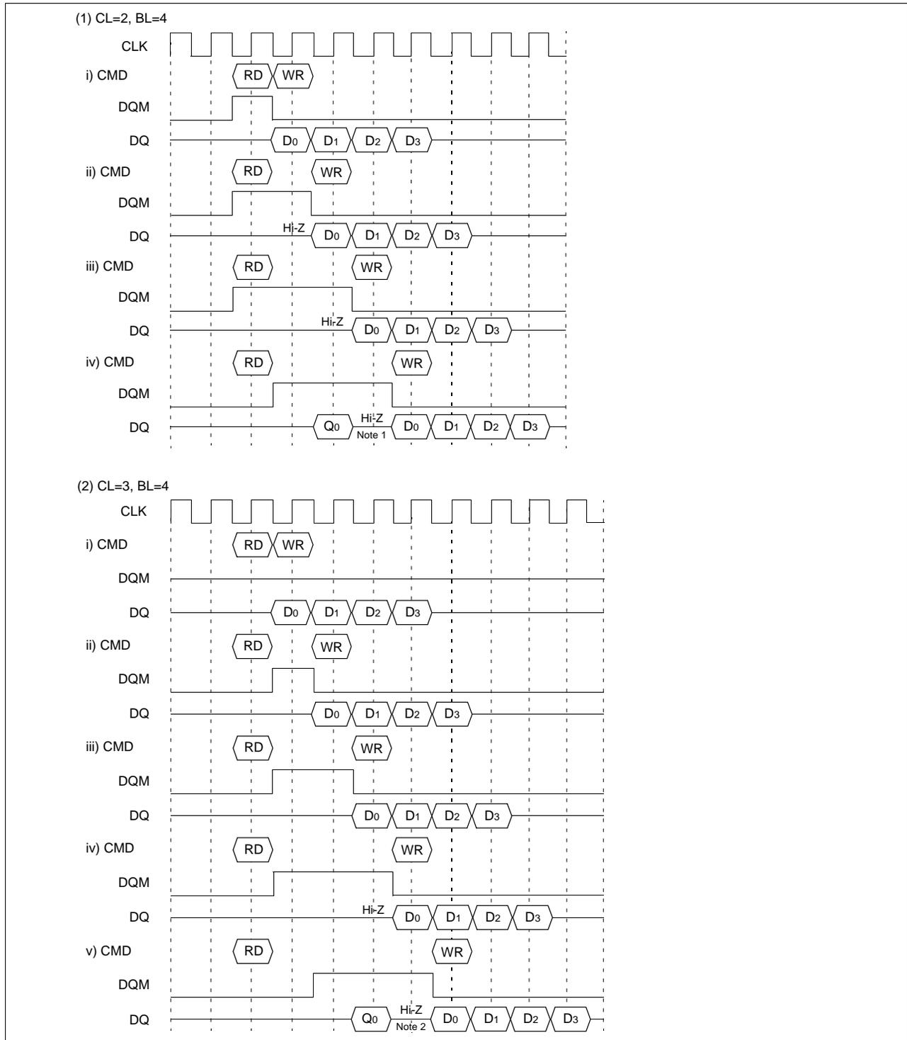
\*Note : 1. To prevent bus contention, there should be at least one gap between data in and data out.
