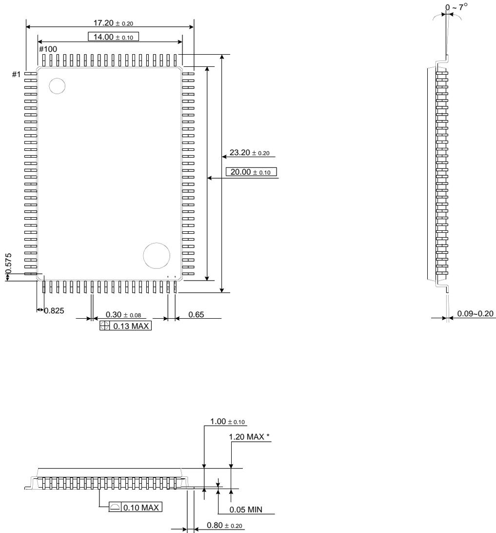
\* All Package Dimensions of PQFP & TQFP are same except Height.
