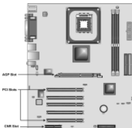
**PCI Slots** PCI slots are used to install expansion cards that have the 32-bit PCI interface.
