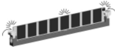
6. Install any remaining DIMM modules.
