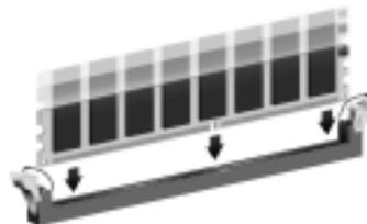
5. Install the DIMM module into the slot and press it firmly down until it seats correctly. The slot latches are levered upwards and latch on to the edges of the DIMM.
