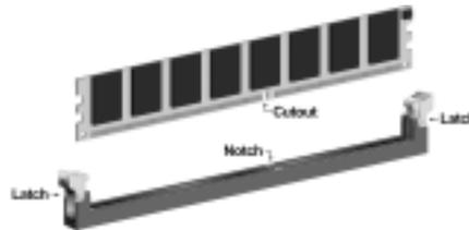
4. Check that the cutouts on the DIMM module edge connector match the notches in the DIMM slot.
